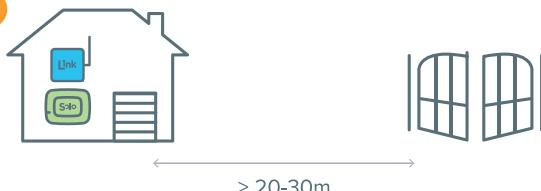
1Control SOLO and 1Control LINK both placed in the house on the window closest to the gate. In this way, taking advantage of the operating range of the remote control copied into your SOLO, it is possible to cover a greater distance and open through the Wi-Fi.
